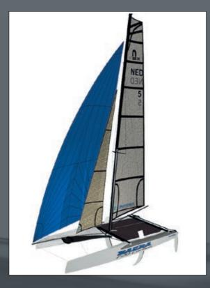
teams the ability to excel! Full carbon hulls, full carbon wing mast profile produced by the same manufacturer as the Olympic NACRA 17 builder Hall Spars, different section in size though.
