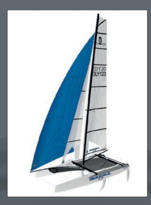
than recent conventional shaped catamarans. This increased stability comes without the drag normally associated with creating high longitudinal stability in conventional shapes, and allows the sailors to push the boat much harder downwind.
