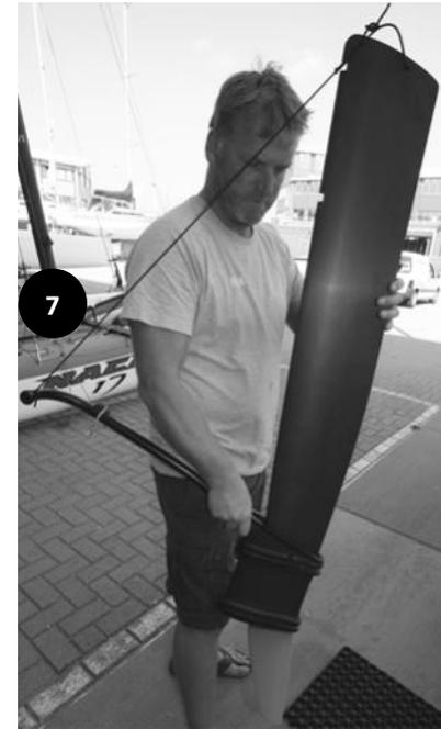
8. Mount the rudderstock on the transom gudgeons using the rudder-pin as illustrated in the figure.
