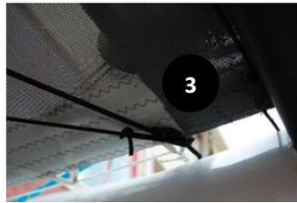
3. Lead the shockcord through the 18mm soft single block diagonal to the forward corner of the trampoline and tie the shockcord to the most forward trampo-
