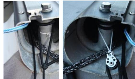
Lead the shockcord through the beam to the otherside, tie the 16mm harken block with the polyester rope to the beam casting to reverse the shockcord back the other entry side and tie on the shockcord to the beam casting.
