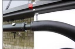
4. Measure the distance between the leading edges of the rudderblade (see A in the illustration below) and compare this length with the distance between the trailing edges. (see measurement B) For good alignment the distances should be equal to each other or facing inwards between 0-2mm. Hence, the trailing edge (measurement B) distance could be 0 to 2mm longer.
