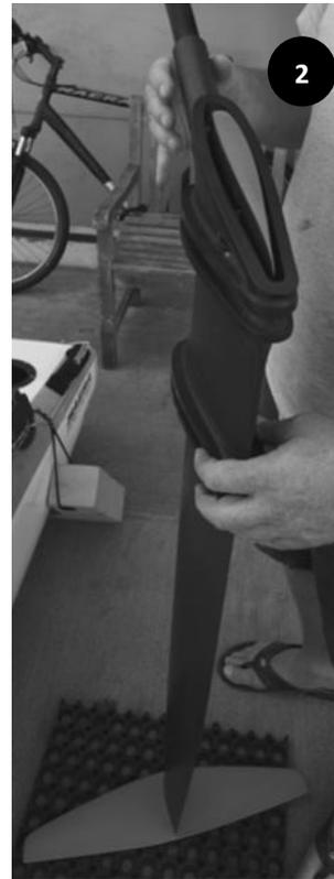
2. insert the head of the rudder foil into the rudderstock cassette.
