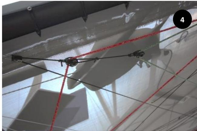
4. Lead the DBD extension lines through the trampoline through the blocks and back through the trampoline as illustrated in the overview. (red and green)
